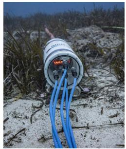
The removal of all individual parts is by design easy, allowing for on-site maintenance or replacement of parts of the system without having to lift out of the sea the entire installation.
