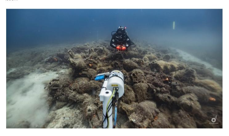
The underwater cameras are digital, colour, state-of-the-art, with high-resolution technology and have a wide-angle lens. Each camera is connected to a local computer, which uses appropriate software to monitor its operating parameters.
