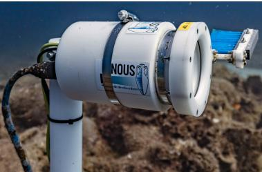
The camera, lens and electronic parts are mounted in a watertight housing (camera housing). The housing is made of thermoplastic, with a removable front part made of transparent crystal and an o-ring seal. The ethernet switch and the fibre-to-copper converter are also located in a sealed hub housing.
